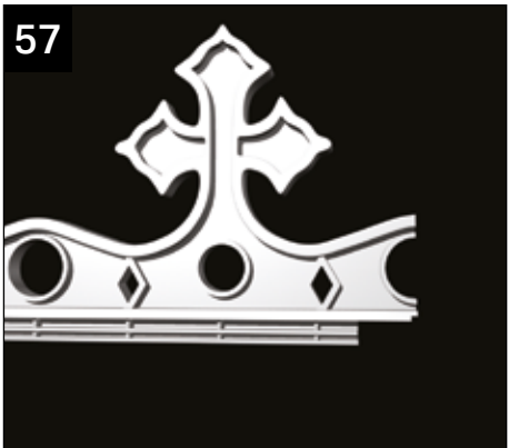
Cut back the underside of the last section of cresting by 40mm.
