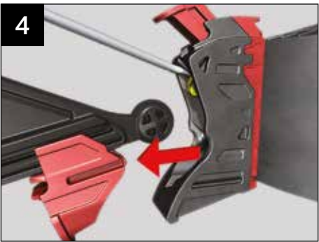
Gently pulling the bar away will automatically release the head of the speedlock.
