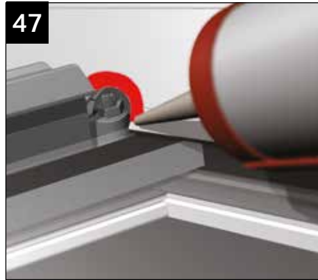
Seal around the notched Georgian top cap ready to receive the jack rafter capping.
