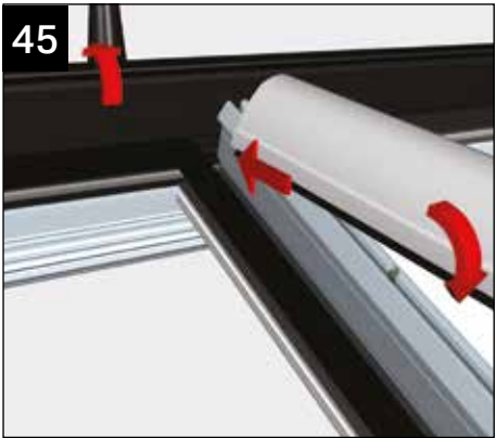
Work your way around the roof. The top cap must be lifted into its final resting place (at the ridge) prior to being knocked down over the Anchor clip.
