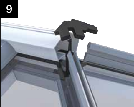
ENSURE THE GLASS IS CLEAN AND DRY BEFORE FITTING. Peel back protective film from weathering shield and position (adhesive face down) on glass, locating around the ridge and the hip bars. Press down firmly. Before installing capping, if jack rafters are specified, please refer to step 45 (page 19) in the Georgian installation
