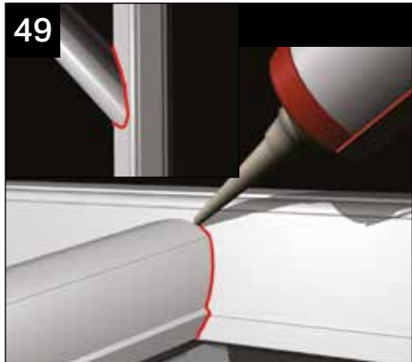
The jack rafter top capping should sit tightly up to the hip bar top capping as shown. Seal around the joint on the jack rafter capping when complete.
