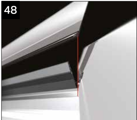
Ensure the jack rafter top capping is lined up correctly (as above) before knocking the top cappings into position. It is not possible to 'tap up' the jack rafter top caps into final position when fitted with anchor clips.
