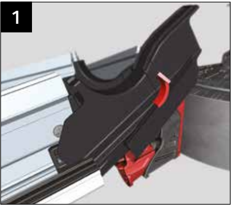
If you need to remove a glazing bar from the speedlock 2 socket assembly, remove the speedlock hood (if fitted) and release and lift the bar at the eaves end.
