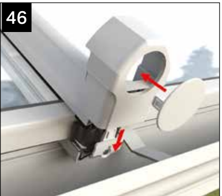
If you haven't fitted already, attach end cap fixing blocks - These arrive attached to the end caps. Fit the glazing bar end caps by sliding onto the fixing blocks. Push fit the insert into the end cap.
