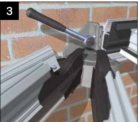
Check the half ridge for being level and then check the starter bar pitch. Drill and fix the die cast back plate to the host wall (avoiding mortar joints) using an anchor bolt suitable for the substrate. Drill and fix the starter bars(s) (as step 24 p12).
